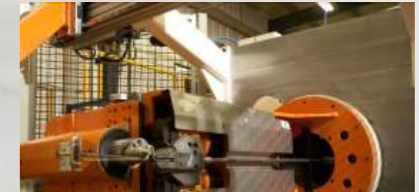
Fully automated wire bending machines process wire from 2.4 to 12 mm.
