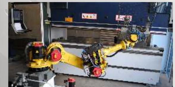
Automated robotic cell cuts and bends wire-mesh with high productivity.
