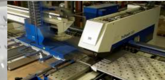
Powerful punching machine works metal from 0.7 mm up to 3 mm thick.
